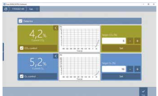
Figure 12: You have full control of the environmental conditions during a run, including the temperature and the CO 2 and O 2 levels inside the reader.
