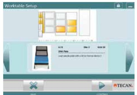
Step by step user instructions help avoid potential errors during worktable setup to ensure correct initial conditions. Then a selection confirmation screen provides a run summary as a final check before the start of the run.
