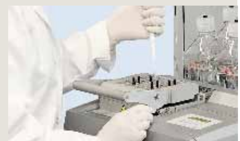
Sample injection using a positive displacement pipette.
