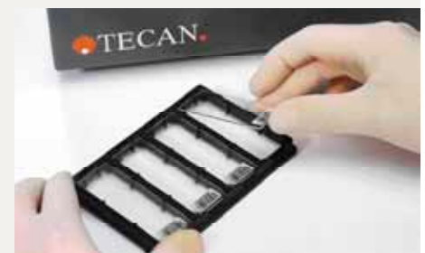
Loading 4 slides at a time on a Tecan slide holder.
